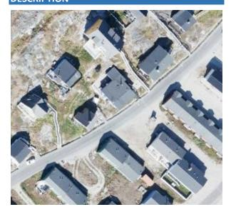
An orthophoto is a composite aerial photo made from overlapping photos that have been geometrically corrected and adjusted to depict equal proportions throughout the image. This ensures uniform scale and prevents elevation variations in the landscape from causing distortions in the image. An orthophoto can therefore be used as a map and linked with a coordinate system.
